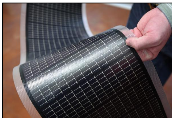
Figure 37: Flexible thin-film PV panel
