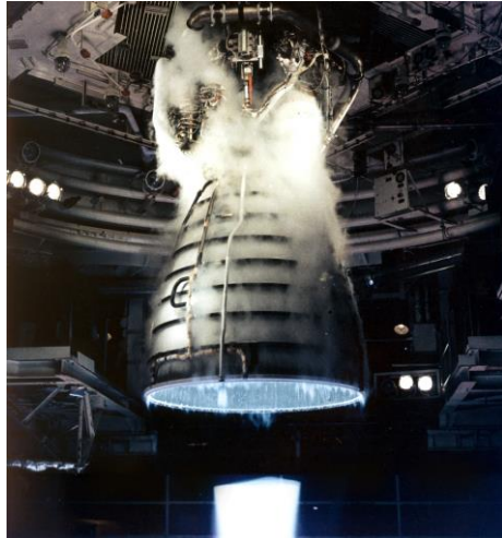
Figure 7: Oxygen-hydrogen combustion in the main engine of a space shuttle.
